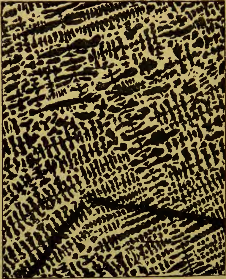
FIG. 15.—Crystals which have separated from a fused alloy of copper and tin ; as seen under the microscope.
